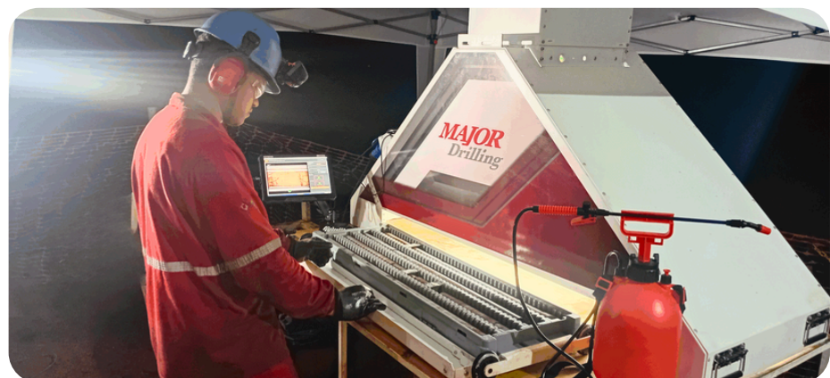
A Major Drilling team member loads core into the Drillside Imaging Unit tray at G Mining Ventures Corp.'s Tocantinzinho Mine.
