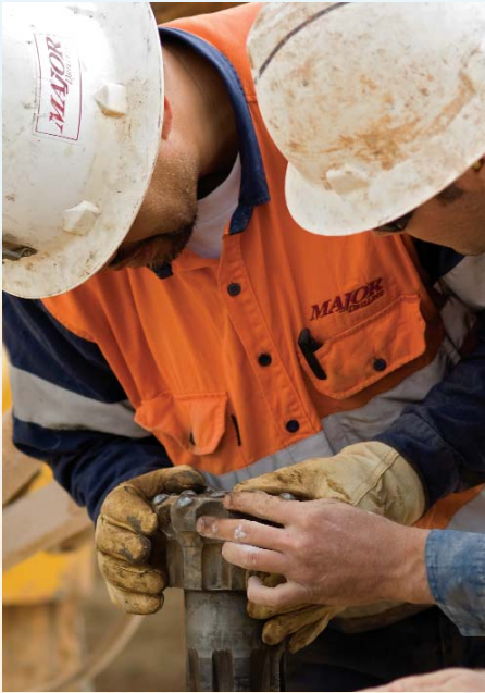
Above: Checking the RC drill bit before drilling begins.
