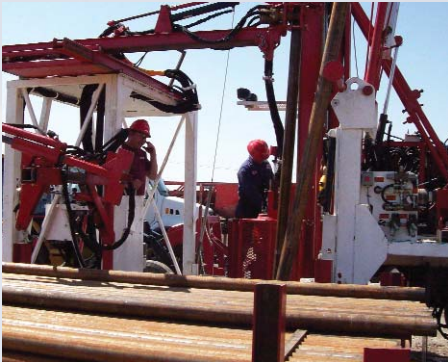
Above: The use of rod handlers improves safety conditions.
