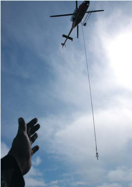
Above: A long line being delivered into the worker's hand.
